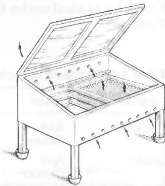
Figure 4.6 Airflow in a cabinet dryer.
