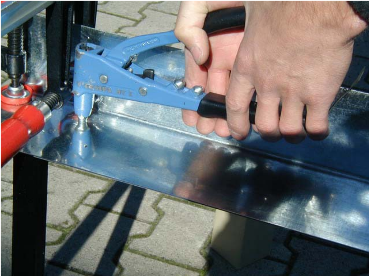
Fig: 14 shows the gripper for blind rivet
