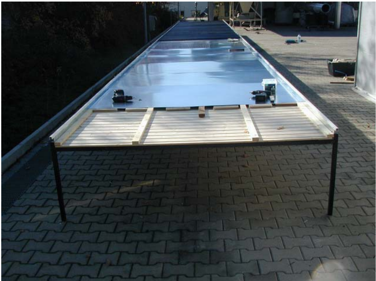
Fig: 43 insert the blank sheet, make sideward holes and screw it on
