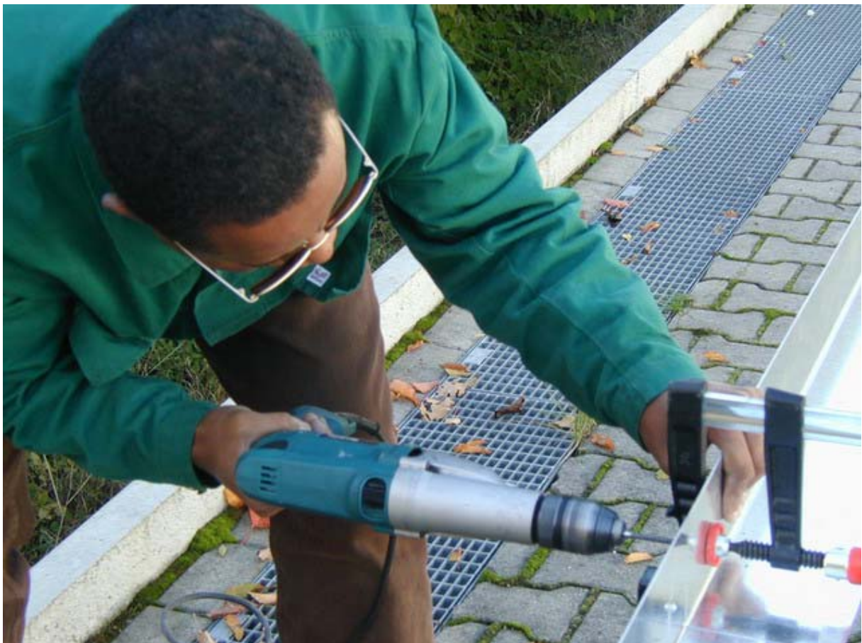
Fig: 4 make holes for rivet in side plate
