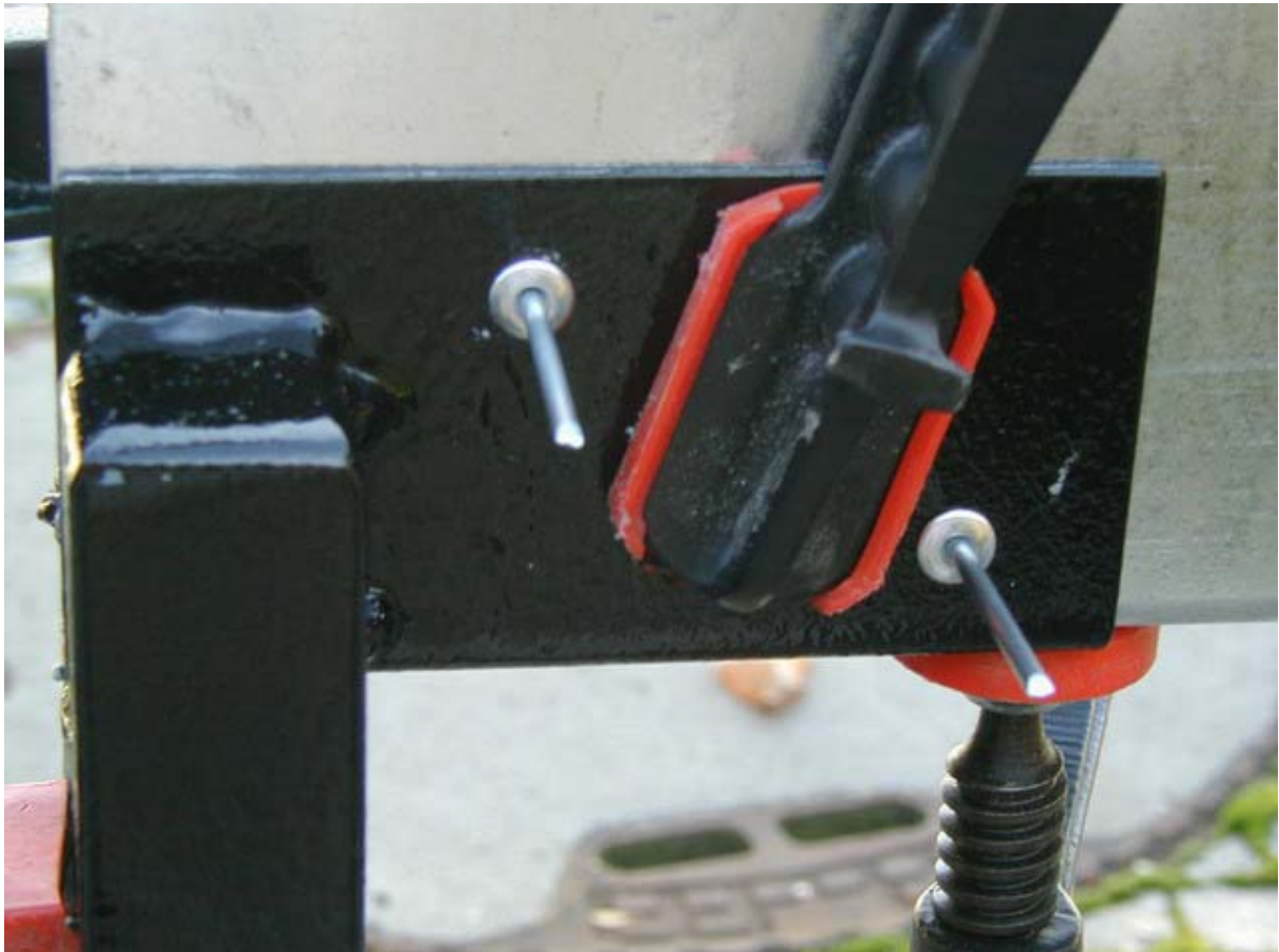
Fig: 6 rivet stick into the holes
