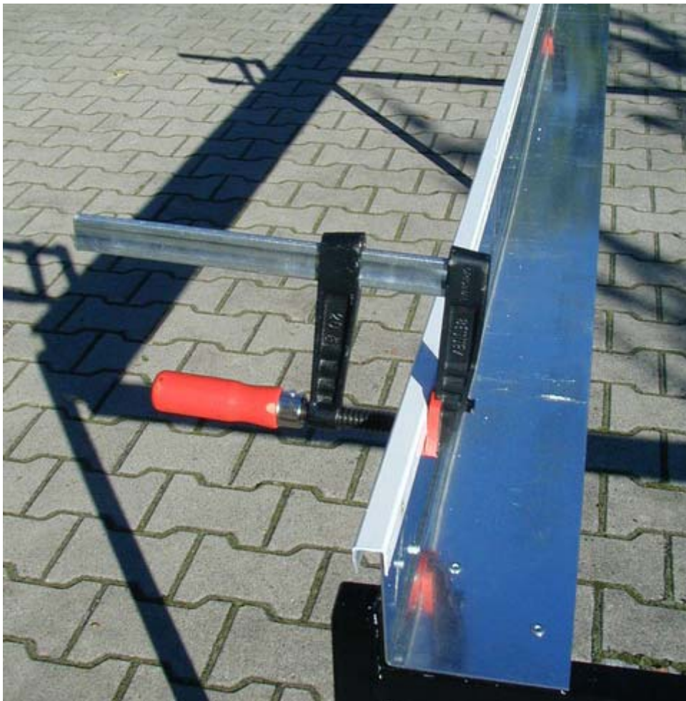
Fig: 17 fix u-profile with a clamp
