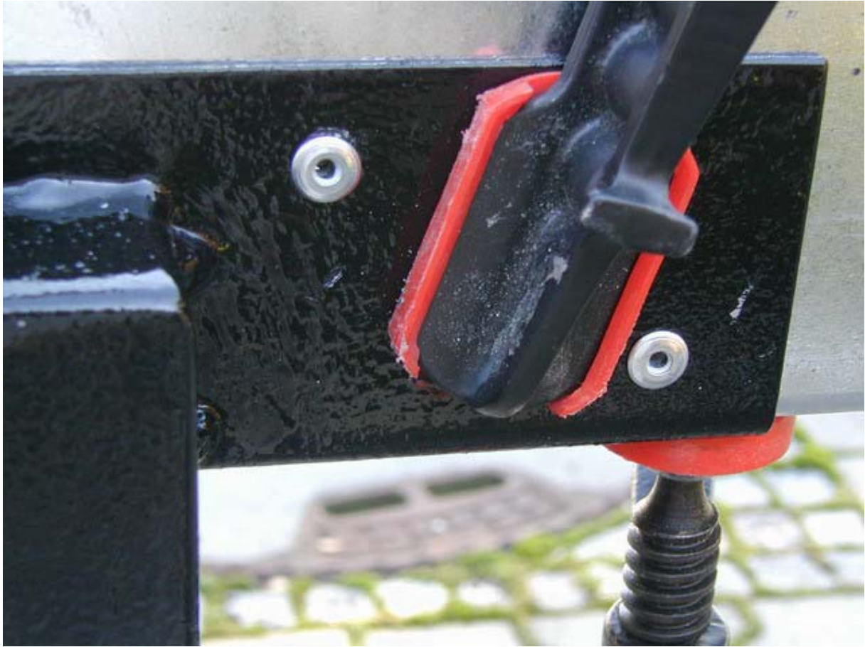
Fig: 7 finished rivet from outside
