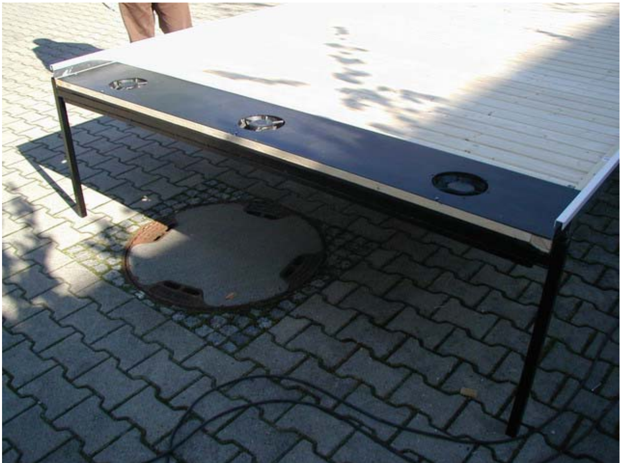
Fig: 30 shows the fan plate built-in the dryer
