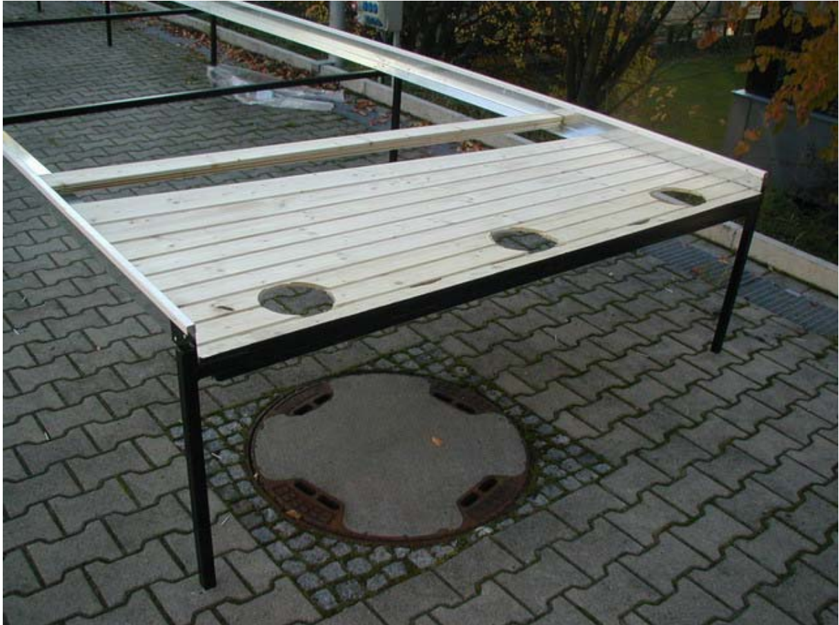
Fig: 21 wooden floor with holes for the three fans
