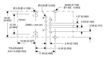
For proper heat dissipation, the PCB should have approximately 1 square inch of copper attached to the shield tabs. The shield tabs are an important source of heat sinking for the device.
