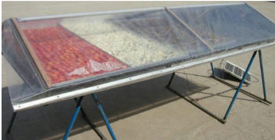
Solar dryer used in India; the base-plate is corrugated roof with aluminum foil on the backside
