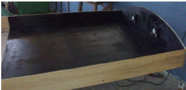
Type of holders for Type 2. You can put the round holders for the Plastic for at least one hour in water to get them bend more easy
